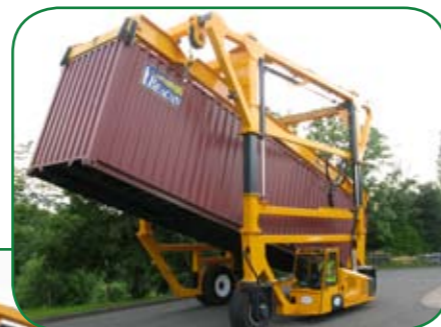
◀ Same Unit can lift 20', 30', 40', 45' Containers
