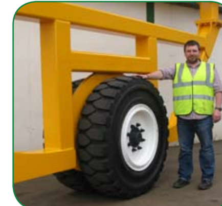
▲ Large Tyres for Low Ground Pressure
