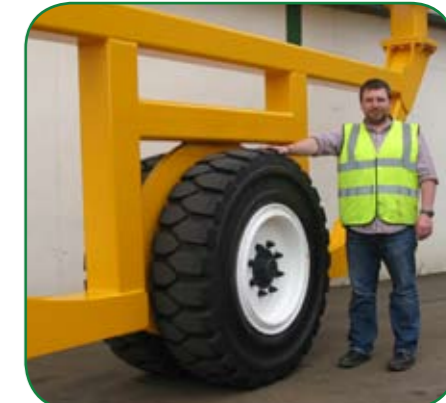
▲ Large Tyres for Low Ground Pressure
