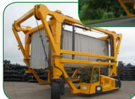
◀ Same Unit can lift 20', 30', 40', 45' Containers
